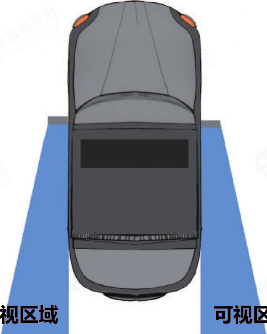
The diagram shows a top-down view of a grey car. Two blue trapezoidal shapes extend backwards from the rear of the car, representing the visible range of the rearview mirrors. The area between the car and the start of these blue shapes is shaded grey, representing the blind spot. The car's rear window is blacked out.
